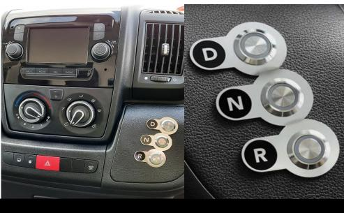
Gear Lever replaced with Drive Mode select buttons located to the left of the steering wheel
